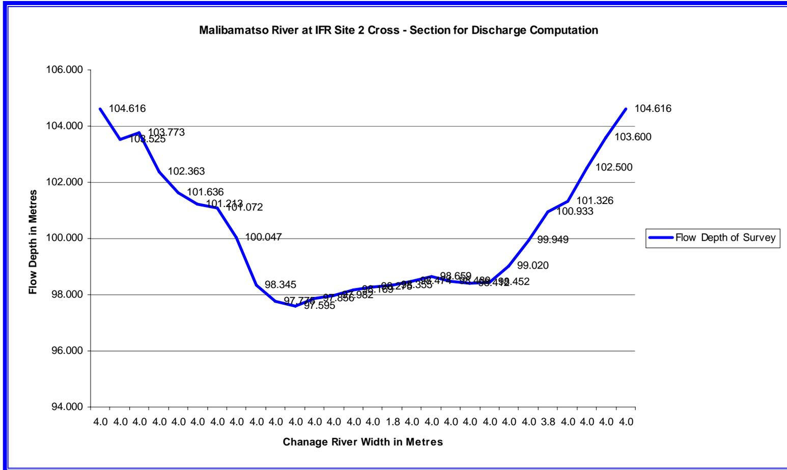
Chart 2 on page 15 presents the actual surveyed cross – section for the Malibamatšo River System at IFR site 2. It is from this graphical presentation where the required hydraulic river flow parameters are easily obtained.
